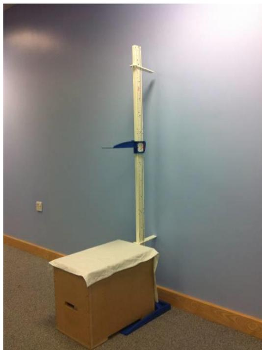
**Figure 2.** Assembled stadiometer mark (first 3 segments) with positioned anthropometric box.
